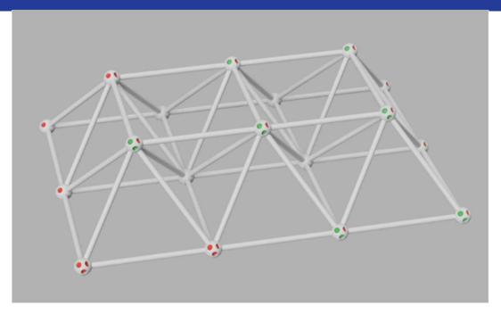
• A standard truss made from 2 meter concrete tubes having an outer diameter of 10 cm and a wall thickness of 1 cm. The pipes are joined by identical spherical concrete nodes into which the pipes are set and cemented.
